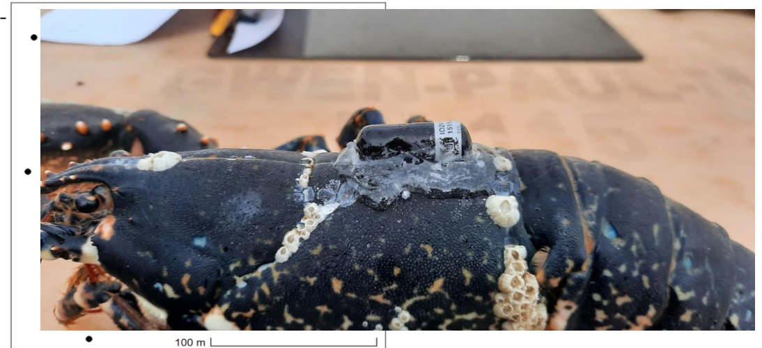
Figure 4: Innoyasea V9 acoustic transmitter attached to carapace of European lobster ( H. gammarus ) using epoxy resin
